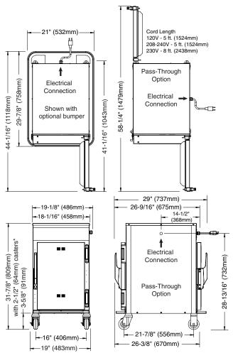
\*33-3/8" (848mm) - with optional 3-1/2" (89mm) casters \*35-1/4" (894mm) - with optional 5" (127mm) casters \*33-3/4" (857mm) - with optional 6" (152mm) legs
